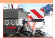
954.V350.LED 1 set Dual-wheel marker board V350 DORA-TP-LED: 2 holders, 2 boards, 1 set of LED lights
